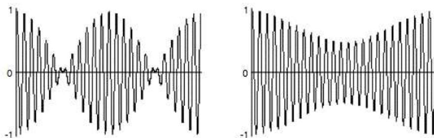
*Ring modulation Amplitude modulation*
