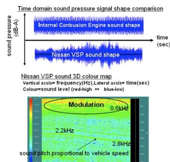
**Figure 1-1. Tabata et al.’s (2011) figure demonstrating frequency content of an ICE, and their synthesized sound.**
